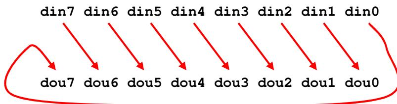
Barrel shifting is shifting by more than one bit. While this seems trivial, when we start looking at synchronous or clocked operations, in some applications it is important to be able to shift by more than one bit in a single clock cycle. Barrel shifting can be either circular or linear.
